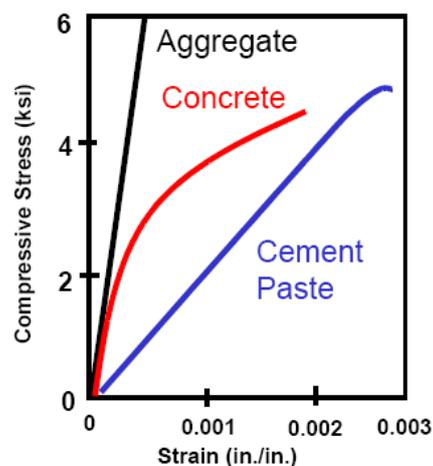
FIGURE 3.1 Stress strain response of behaviour of concrete (1 ksi = 6.89 MPa).
